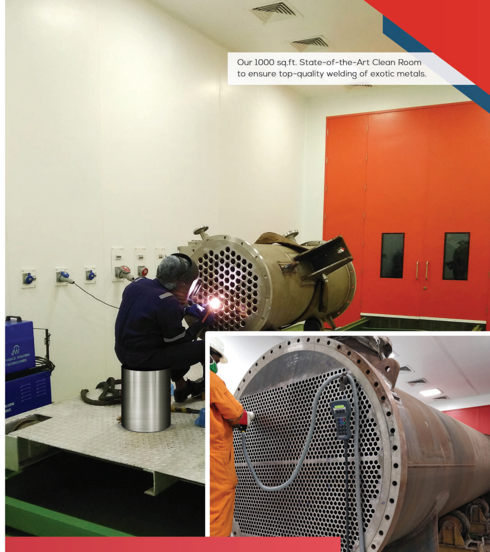
Orbital Welding of Titanium Tube to Tubesheet Joint
