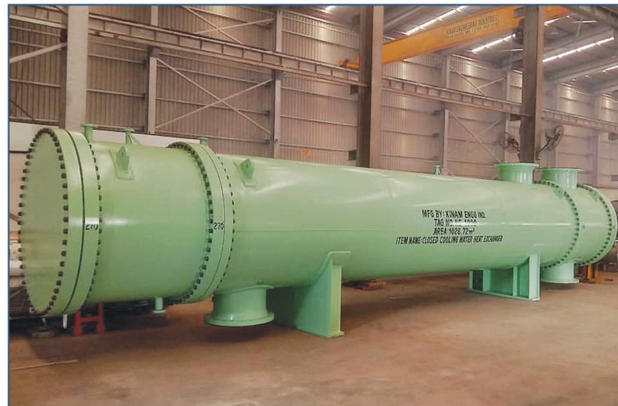
Closed Cooling Water Heat Exchanger 1028 m 2 made of Titanium
