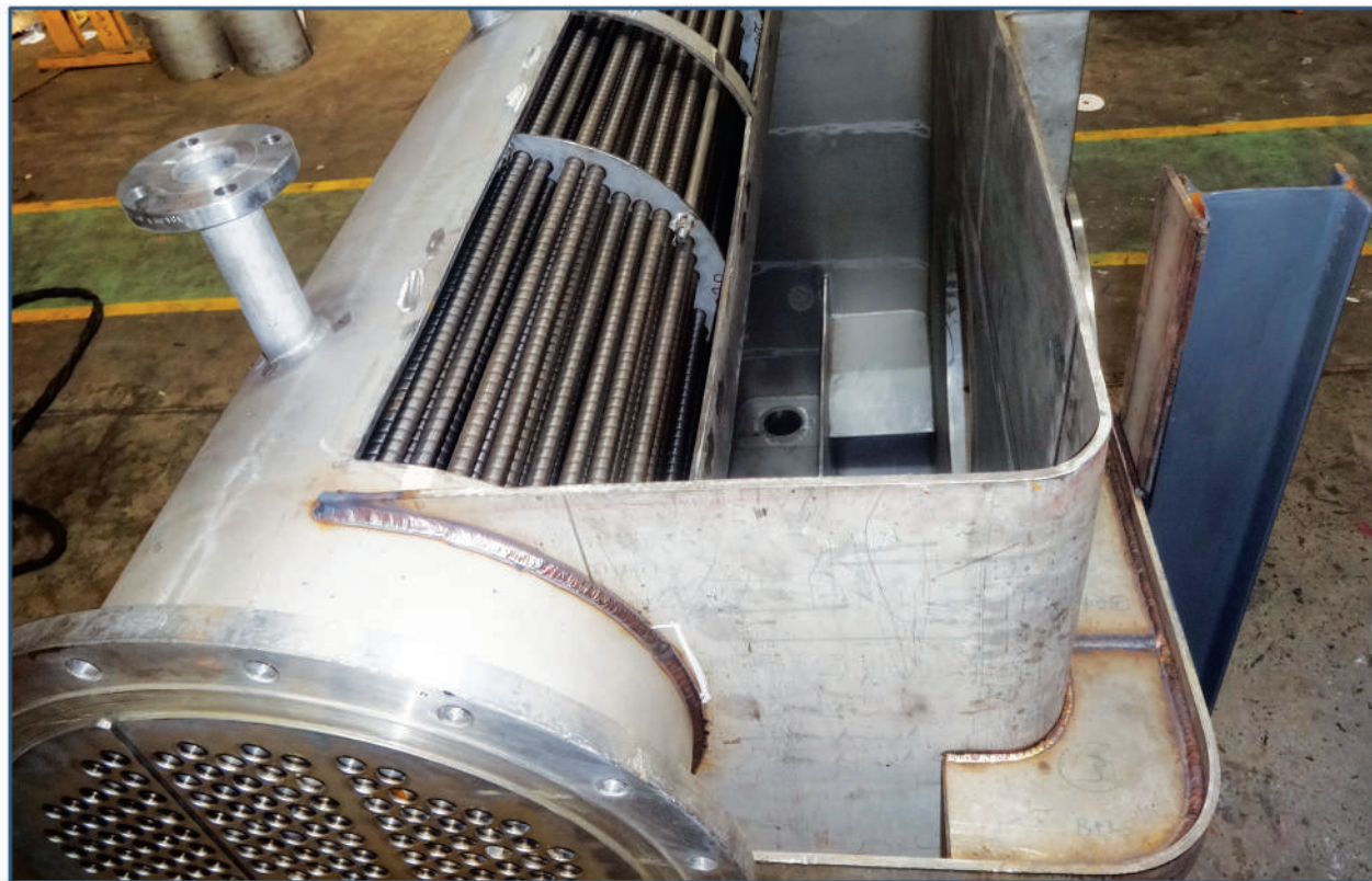
Titanium Corrugated Tube Heat Exchanger for De-salination Pilot Plant
