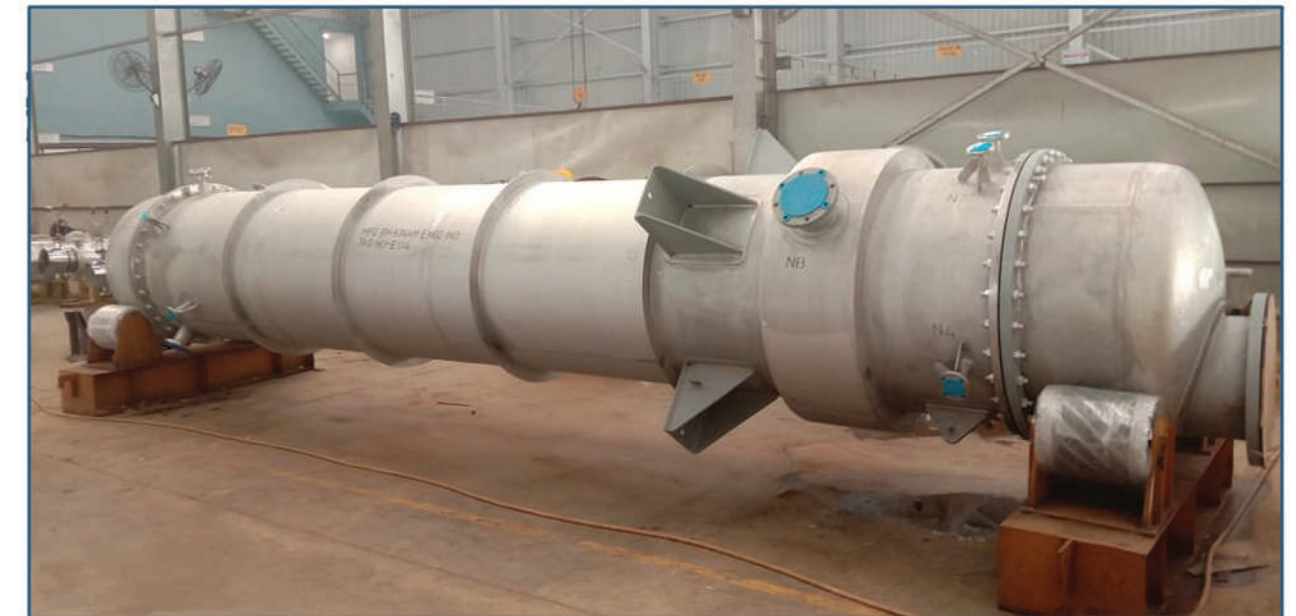
Duplex Heat Exchanger with Titanium Tubes
