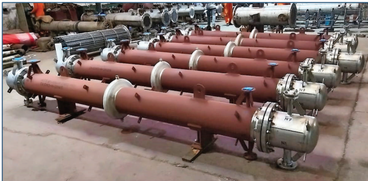
C-22 Condenser with Corrugated Tubes
